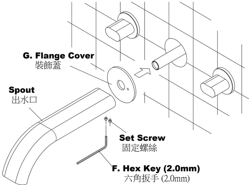
\* Put **Flange Cover** between Spout and Finished Wall, insert **Spout Connector** into **Spout** and align with **Flange Cover**, and then tighten **Set Screws** underneath **Spout** with **Hex Key(2.0mm)**.
