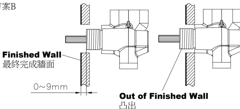
\* Suggestion A: Please screw the **Long Type Extension Connector** into the **Handle Assemblies of Hot and Cold**.
