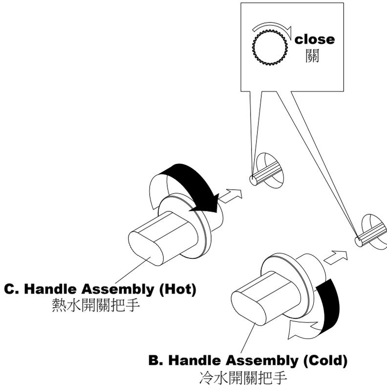
\* Turn **Hot Valve** and **Cold Valve** clockwise to closed position before installing the **Handle Assemblies**. Screw both **Hot and Cold Handle Assemblies** with **Extension Connectors** to the threaded shanks of valve securely till against the wall.
